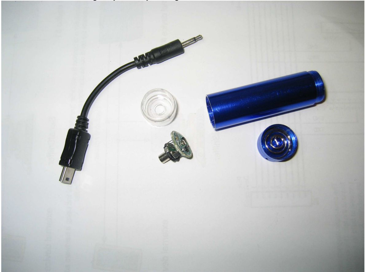
The dismantled Emergency Battery Charger
